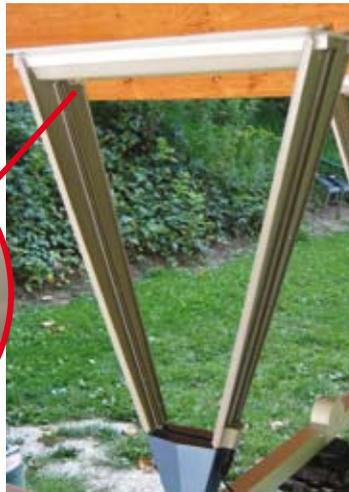
the light over the Start Sensor. This causes the M2 chronograph to start timing. As the arrow travels over the M2 chronograph sensors, the arrowhead eventually reaches the Stop Sensor. This causes the M2 chronograph to calculate and display the velocity. The M2 chronograph now takes a short amount of time to reset and get ready to capture the next Start Sensor event. (The M2 chronograph does this very rapidly as it is designed to capture velocities from automatic weapons.)
